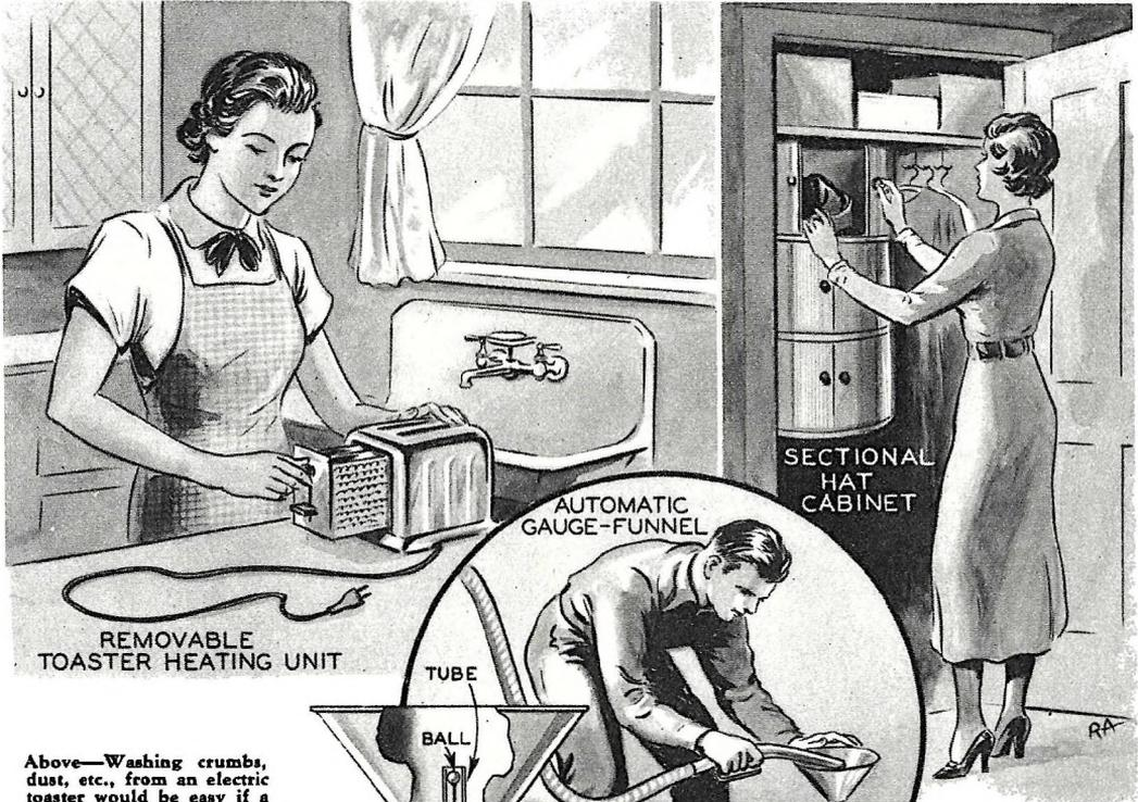
Above—Washing crumbs, dust, etc., from an electric toaster would be easy if a removable heating unit was developed. Short circuits would be avoided since outer case could be thoroughly dried before replacing heater. Right—Thousands of filling station operators would welcome a funnel with built in gauge. It would eliminate messy, wasteful overflow.
