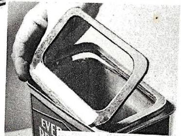
Cut from two pieces of plywood hinged frames, at right, are installed half way inside the can. Yellow filter paper is attached to the smaller frame.
