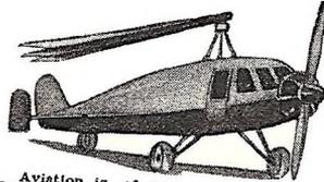
Aviation is, of course, a fertile field for inventive ingenuity. Important steps have been made to bring about the plane which average Mr. American man and woman can fly. Shown is an improved type of autogyro designed to land in any convenient spot. Then wings fold back and the plane serves as an automobile. Just one of many unusual aeronautical developments during the past year.
