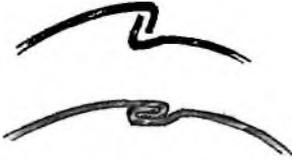
The hooks are brought together and pressed to form the seam. The extra thickness is inside the container.
