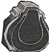
Many advances have been made in tire construction. Shown is a new Life Guard Tube introduced by Goodyear. Has a secondary tube within a main tube. Many other developments in tire construction have taken place.
