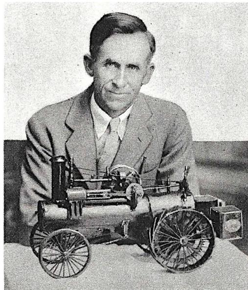
L. K. Woods, of Mendon, Utah, owns the oldest steam traction engine in the Rockies. He built this working model of it which weighs 26 pounds and is 19½" long, 11½" high.
