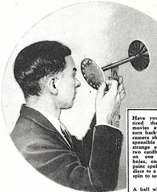
Have you ever noticed that in the movies auto wheels turn backward? The camera shutter is responsible for this strange effect. Cut two cardboard discs: on one cut peep holes, on the other paint spokes. Attach discs to a handle and spin to see the effect.
