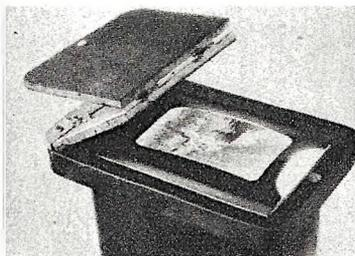
Completed printing platen is shown at right with a negative mounted over the printing glass. The plywood backing is hinged in two places and dark felt glued to the back to provide a light tight surface.
