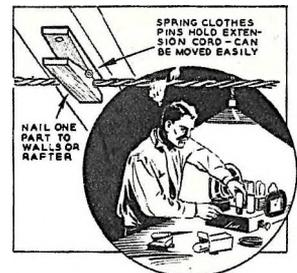
Spring clothes pins attached to the walls and ceiling of workshop are useful for holding extension cords.
