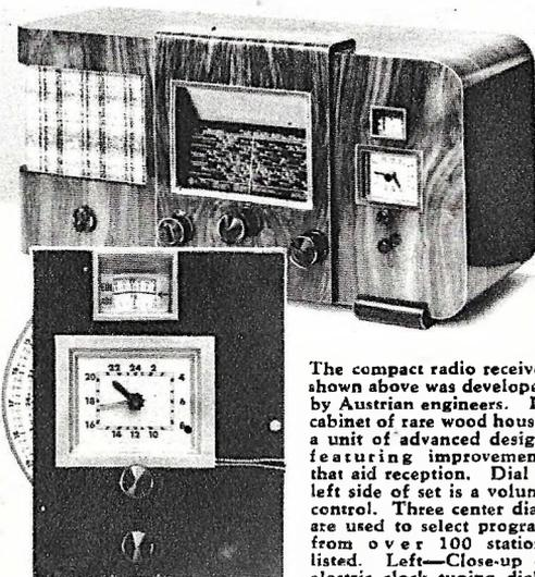
The compact radio receiver shown above was developed by Austrian engineers. Its cabinet of rare wood houses a unit of advanced design, featuring improvements that aid reception. Dial at left side of set is a volume control. Three center dials are used to select program from over 100 stations listed. Left—Close-up of electric clock tuning dials.
